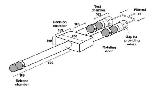
(*Part 2*) Implement the use of sensors within the olfactometer to automatically log the amount of mosquitos flying into either test chamber. There are no restrictions on sensors/cameras used for detection. Data collected must be logged and stored in an easily accessible way.
