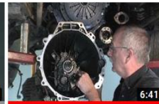
Servicing Quick Connect / Quick Disconnect Pull Type
