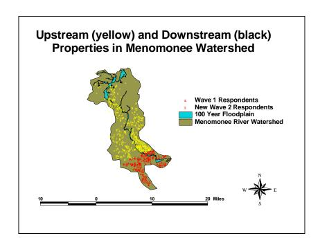
ArcView was programmed to determine the unique flood risk, as defined by the recurrence interval (i.e., the expected years between flooding events from the Menomonee River for the property) for individual properties within the watershed. Since much of the flooding within the Menomonee River watershed was in the region from the Village of Wauwatosa to the southeast, ArcView was also used to identify upstream and downstream properties.
